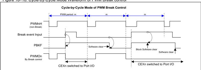
Bit 4~3: PBKE1.1~0, PWM Break Enable 1 selection. This function is only active on CEXn output mode (n=0~5).
