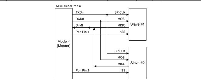
The SPI master satisfies the transfer with the full function SPI module of Megawin MG82/84 series MCU with CPOL, CPHA and DORD selection. For CPOL and CPHA condition, **MG82G5E32** uses an easy way by initialize SPI clock polarity to fit them. Table 18–12 shows the serial port Mode 4 mapping with the four SPI operating mode.
