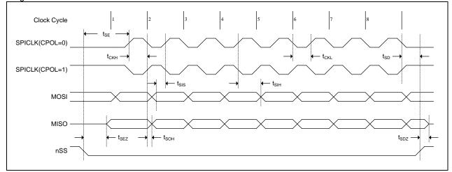
Figure 34-6. SPI Slave Transfer Waveform with CPHA=1
