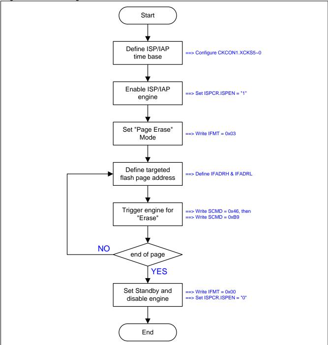
Figure 29–3 shows the demo code of the ISP/IAP page erase operation.
