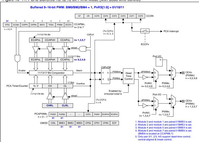
Figure 16-11. PCA0 Buffered 10/12/16-bit PWM Mode (with dead time control)
