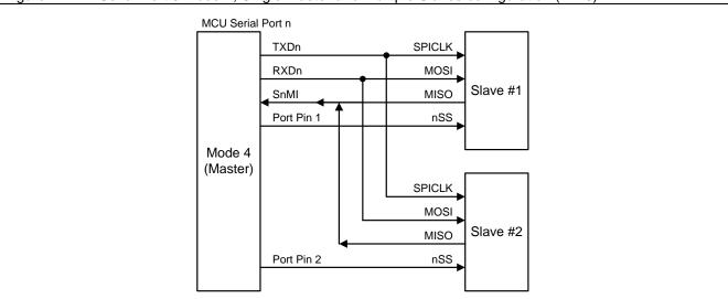
The SPI master satisfies the transfer with the full function SPI module of Megawin MG82/84 series MCU with CPOL, CPHA and DORD selection. For CPOL and CPHA condition, **MG82G5E32** uses an easy way by initialize SPI clock polarity to fit them. Table 17–39 shows the serial port Mode 4 mapping with the four SPI operating mode.
