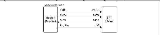
Figure 18–3. Serial Port 1 Mode 4, Single Master and Multiple Slaves configuration (n = 1)
