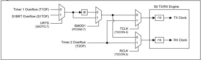
When S1 is used as the baud rate generator, the baud rate is as follows.
