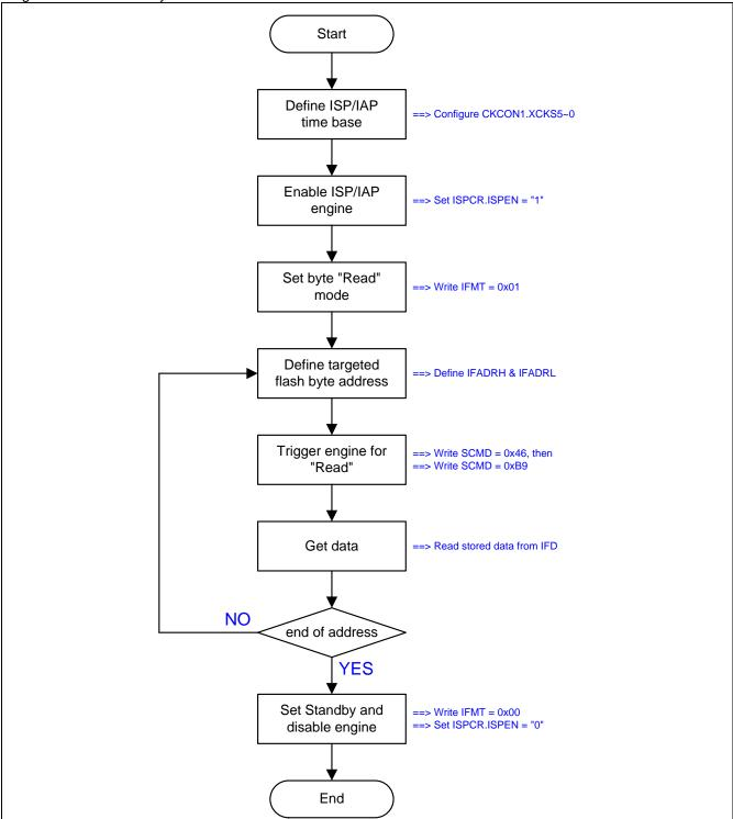
Figure 29–7 shows the demo code of the ISP/IAP byte read operation.
