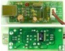
Access ST3679 data to PC using this board, It installs virtual COM port on PC to which any terminal software can connect.
